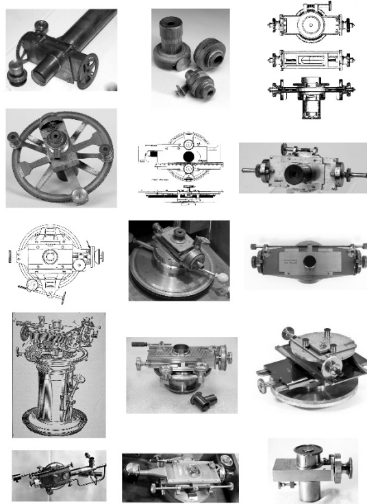
Fig 1: Micrometer designs: Top Row – Smeaton (1770), Nairne & Blunt (1780), Troughton (1795); 2nd Row – Dollond, Amici, Dollond; Middle Row – Fraunhofer (1820), Schroeder, Cooke; 4th Row – Repsold (1860), Clark, Grubb (1885); and Bottom Row – Burnham, Warner & Swasey (1896), Watson (1915).
